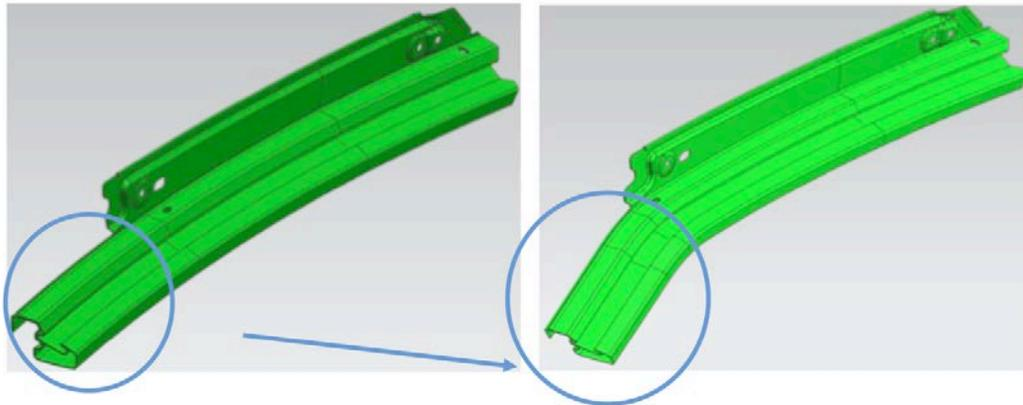
It was an extremely challenging part with varied cross-sections along with rolling, flanging, punching, trimming and bending involved in the molding process. Wang assisted them to set-up the simulation and evaluate the results. Hailed as the leader in accuracy, the simulations yielded extremely accurate correlation results when compared to the final part. The actual result compared with the early simulation result was within 1%.
